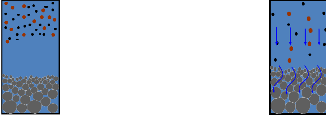
Figure 5. Backwash flow is stopped and media allowed to settle. Wastewater containing high concentrations of suspended iron and manganese flocs is decanted. The cleaned filter is placed back into production.
